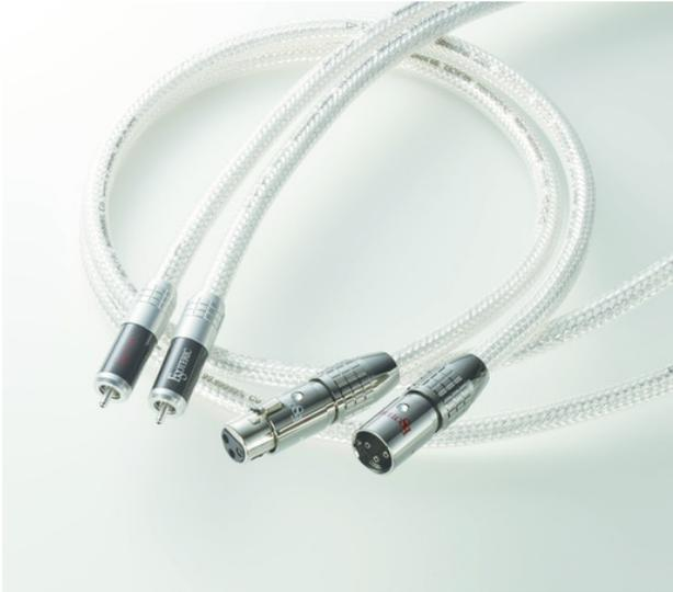
The 7N-DA6300III MEXCEL is the flagship balanced cable in the MEXCEL cable line. It has thick, twin 1.6 mm solid MEXCEL center conductors and triple-layer shielding. (Pure silver plated 7N Cu ultra-thin flat wire braid + copper Mylar tape + thick silver-coated Cu braid)
