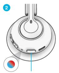
Press and hold button for **8 seconds.** Release. Lights will **flash blue/red.**
